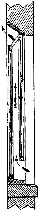
SECTION WITH SASHES DOWN
