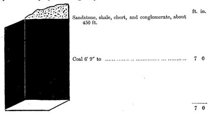
Section showing the thickness and character of the coal-seam newly opened out and worked by the Centenary Coal Co. at Curlewis, in the county of Pottinger. The coal is of excellent quality, and is worked from an adit situated 2 miles 4 chains from the Curlewis Railway Station. The Company have secured the Government railway contract for 1889. The seam has a slight dip north 60 west, and is about 1,220 feet above sea-level.
