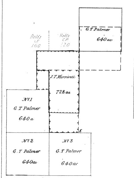
G.T Palmers 640 ac as measured edged blue on Organial as described edged red. On tracing as measured shown by a hold line thus as described by a broken line thus
