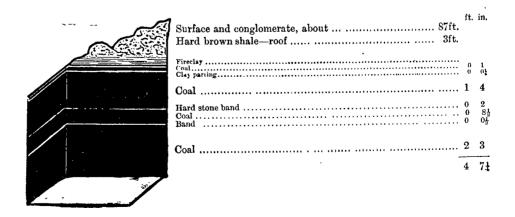
Section showing thickness and character of the bituminous coal-seam lying 60 feet above Deihm's Kerosene Vale coal-seam, opened out by an adit by the Cullen Bullen Coal Company, at Cullen Bullen, in the county of Roxburgh. The Company are thinking of making coke from the 3 feet 1 inch of bituminous coal at the bottom of the seam.
