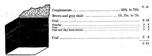
Section of the seam of coal, lying above the Burwood seam, worked at Fern Valley Collicry, on Messrs.
